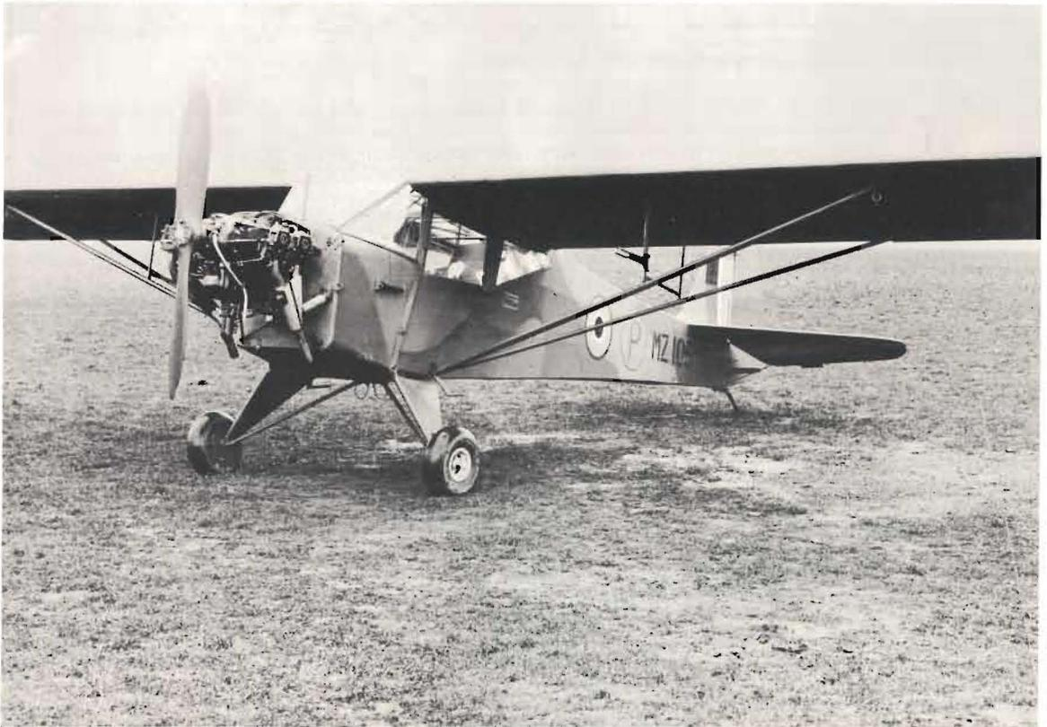
The first prototype Auster AOP.2, MZ105 is seen posing for official photographers, and displaying its Lycoming engine. Of interest in this view is the tail-skid and the 'P' marking, signifying a prototype. (Crown Copyright)
